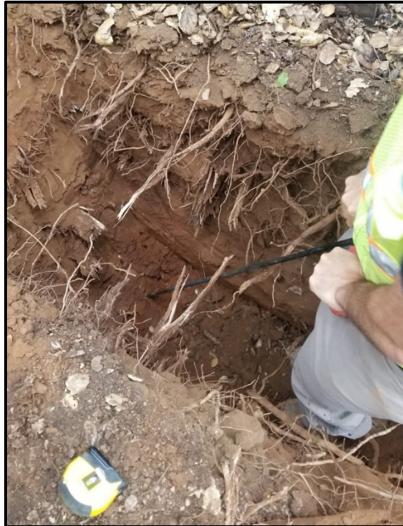
Figure 4-3. Unit 2 Residual Soil, In-Place Probing
